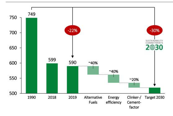
Specific net CO<sub>2</sub> emissions: kg CO<sub>2</sub>/t cementitious material
